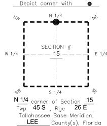
FOUND BASE OF 1-1/2"X2" LIGHTER WOOD POST WITH TACK IN TOP FLUSH WITH GRADE.
