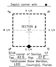
FOUND 1/2" IRON ROD IN CUT-OUT 0.45' BELOW ROAD SURFACE 1.7' SOUTH OF S.R. 78 CENTERLINE
