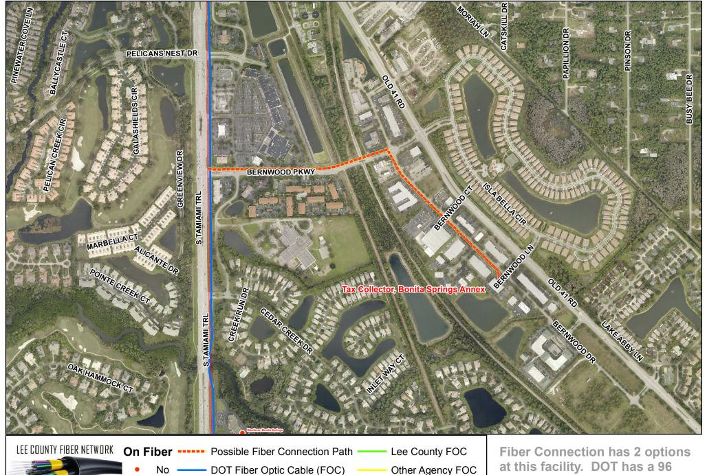
Yes —— ITG FOC **FPL Fiber Facilities** Footage | Cost - Conduit & Fiber Install | Conduit Available | Cost - Fiber Pull | Nearest Connection **County Facility** \$19,474.76 DOT/FPL Fibernet 3,895.0 \$101,268.75 No Tax Collector, Bonita Annex
