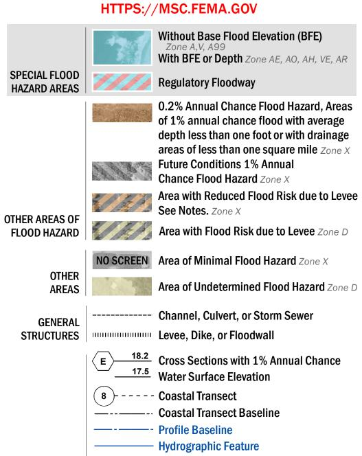
**Base Flood Elevation Line (BFE)**
